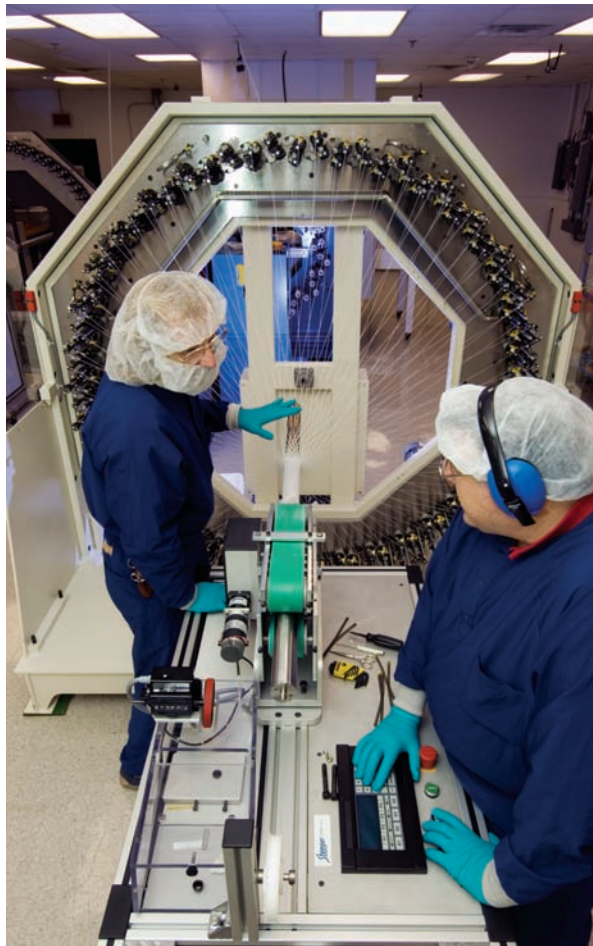
Engineers demonstrate braiding (the intertwining of three or more yarns), a technique to make fabrics for various medical device applications.
