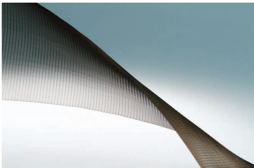
A woven metal fabric, made from a monofilament nitinol wire. The fabric was annealed to maintain a uniform pore size throughout.
