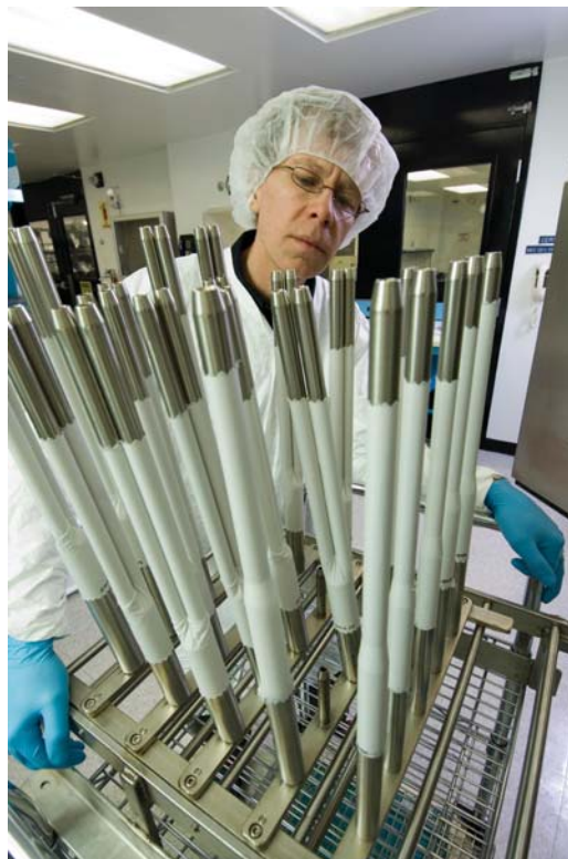
A technician prepares woven polyester grafts for annealing. This seamless tubular fabric is woven flat, cleaned and then placed over mandrels for heat-shaping to produce a 3D structure.
