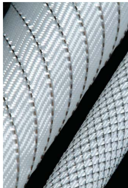
The woven tubes are made with polyester and a reinforcing Nitinol wire. The smaller tube has reinforcing wires in opposite winds to prevent kinking.
